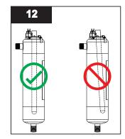
• Ensure quartz sleeve is properly centered in the chamber.
