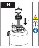
Insert new lamp into the quartz sleeve and thread into sleeve bolt until hard stop.
