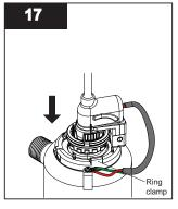
Align connections by rotating ring clamp to push lamp plug onto end of lamp.
