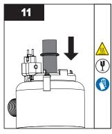
• Place O-ring on the sleeve as shown. Insert the sleeve into the chamber as shown in step 12.
