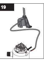
Connect the green ground wire and red strain relief wire to the chamber using the grounding screw.
