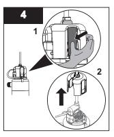
• Remove the safety cap by squeezing the tab.
