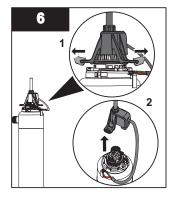
Remove the lamp connector by pulling the tabs out and then upwards.
